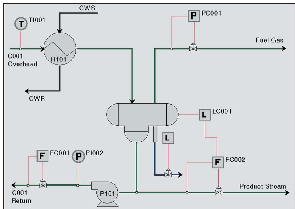
In this example, the plant has experienced an unexpected loss of flow between the discharge of the pump and the downstream process equipment. The loss of flow could be caused by a variety of problems including but not limited to incorrect valve line up, pump failure, valve malfunction or line plugging.
